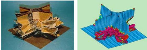
Figure 9. A failed composite cruciform energy absorbing structure (left) and PAM-CRASH model (right) [12].
