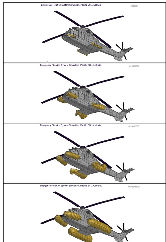
Figure 5: Inflation of the EFS on a helicopter.
