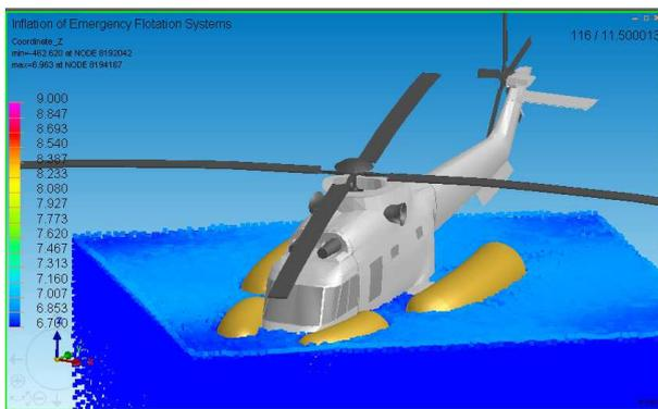
Figure 6: Generic Helicopter with inflating flotation devices.
