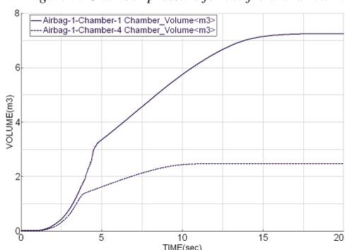
Figure 4: Chamber volume for the front and rear EFS.
