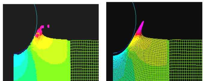
Figure 1: A segment of the FE (left) and SPH and FE (right) simulations in PAM-CRASH. Contours indicate velocity magnitudes, showing good correlation with each other.
