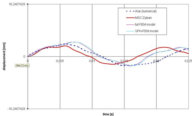
Figure 2: Time history of the deformation of the cylinder bottom for the FE simulation (purple) and SPH model (light blue) vs. the numerical results from Arai and Bereznitski (MSC-Dytran) for a drop height of 0.75 m.
