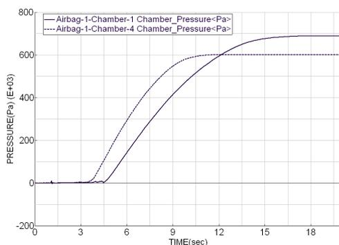
Figure 3: Chamber pressure for the front and rear EFS
